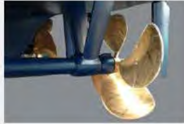
Enclosed propeller shaft and rope cutter
