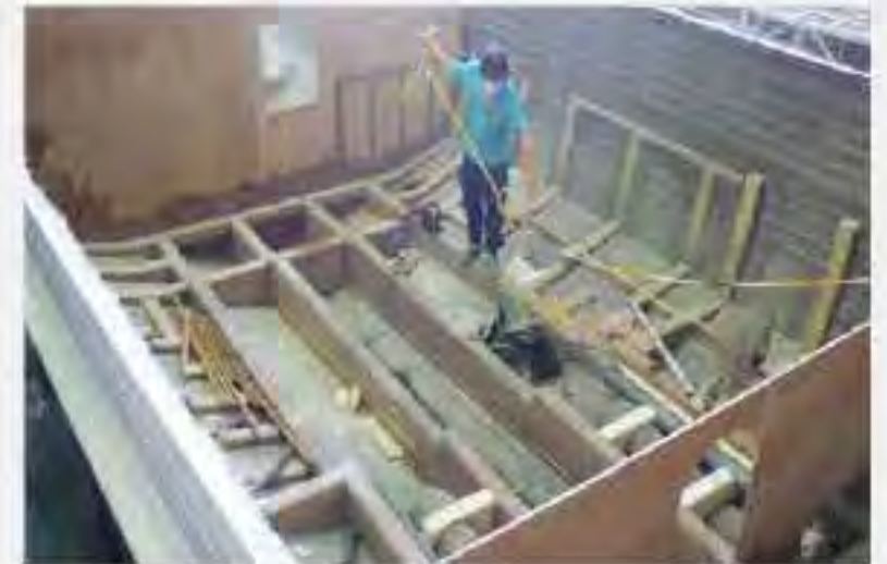
Interlocking Frames and Stringers
