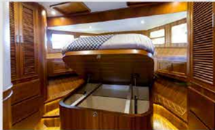
Master cabin bed lifts at the press of a button to reveal large storage area. The bed also slides aft to make changing the sheets easier
