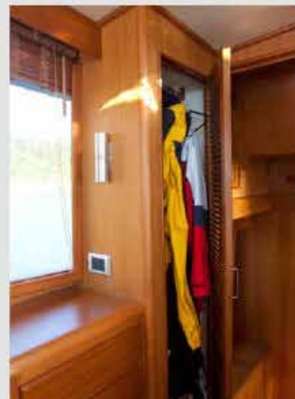
Wet locker in pilot-house is vented and drained overboard
