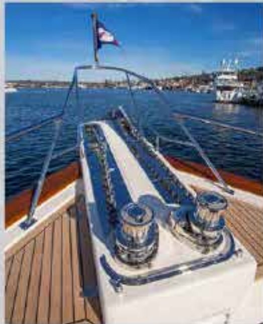
All Fleming's are equipped with two independent windlasses for redundancy
