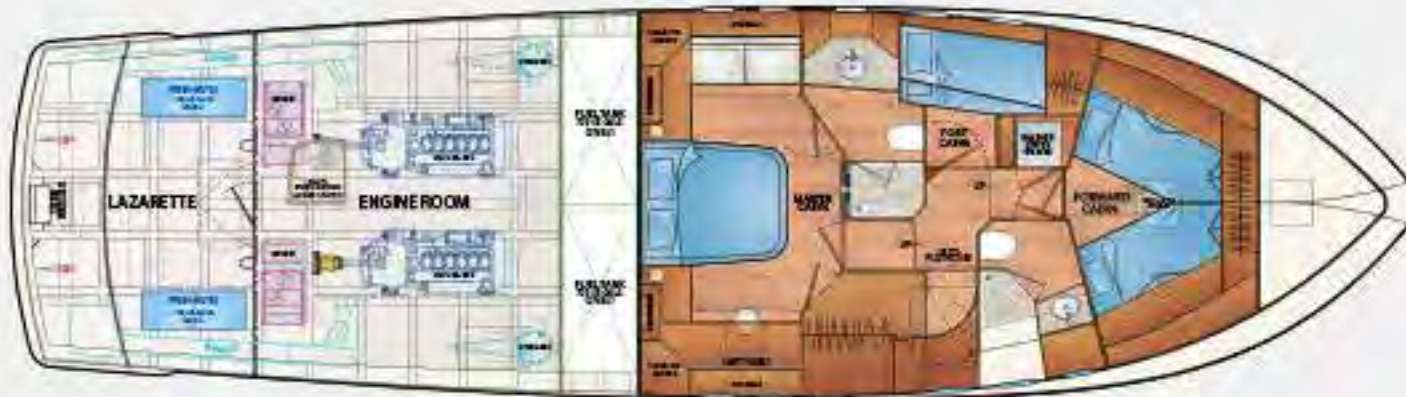
FLEMING 58' – ENGINE ROOM with ACCOMMODATION – OPTION C
