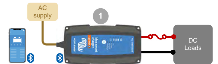
Blue Smart IP65 battery charger used as a power supply.
